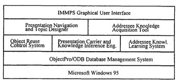
Figure 1: The software architecture of IMMPS
