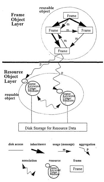
Figure 3: The database hierarchy consists of two layers
